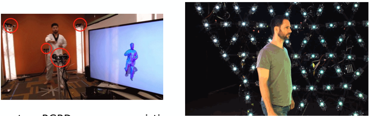
8 custom RGBD cameras consisting of 24 individual cameras.
