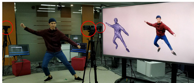
Fig. 1. Illustration of the system setup and the real-time reconstruction results of our UnstructuredFusion. The red circles indicate the unstructured sparse multi-view RGBD cameras.
